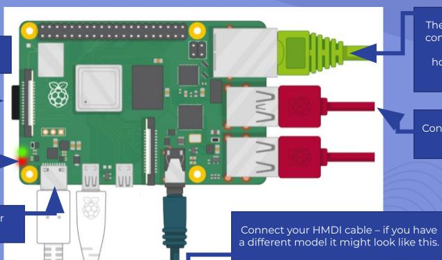
The ethernet port is where you might connect your ethernet cable (used for wifi) – if you have a wifi dongle however, it will fit in one of the USB ports.
