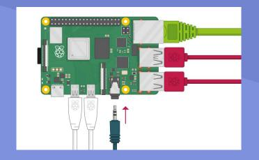
Your Raspberry Pi doesn't have a power switch: as soon as you connect it to a power outlet, it will turn on.
