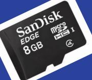
A micro SD card, preloaded with NOOBS or installed with the most recent version of Raspbian.
